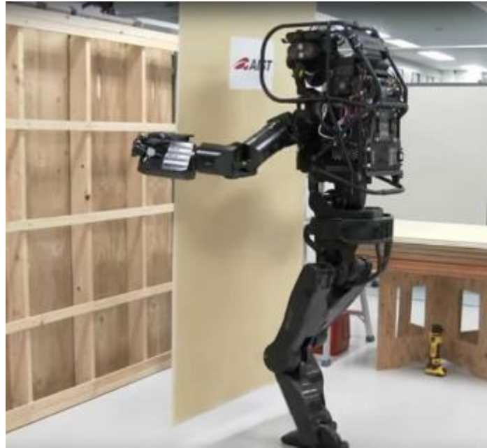
Japanese plasterboard robot
