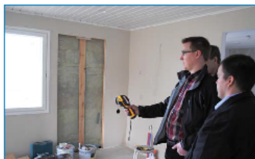
Observing the critical points for the energy efficiency with the infrared camera for leaks in the mantle of the building. Build Up Skills Finland workshop in May 2012.
