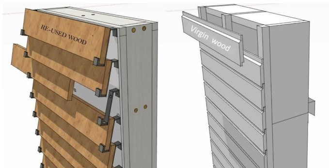
HOOK VS NAIL CONNECTION
