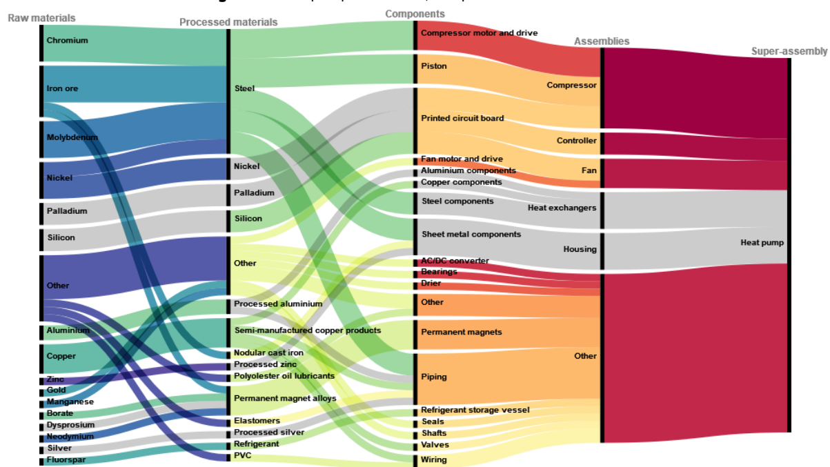
Figure 3. Heat pumps materials, components and assemblies
