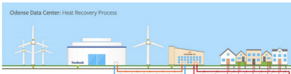
Figure 6 – Integration of waste heat (data centre) within an existing DH system (Fjernvarme Fyn)
