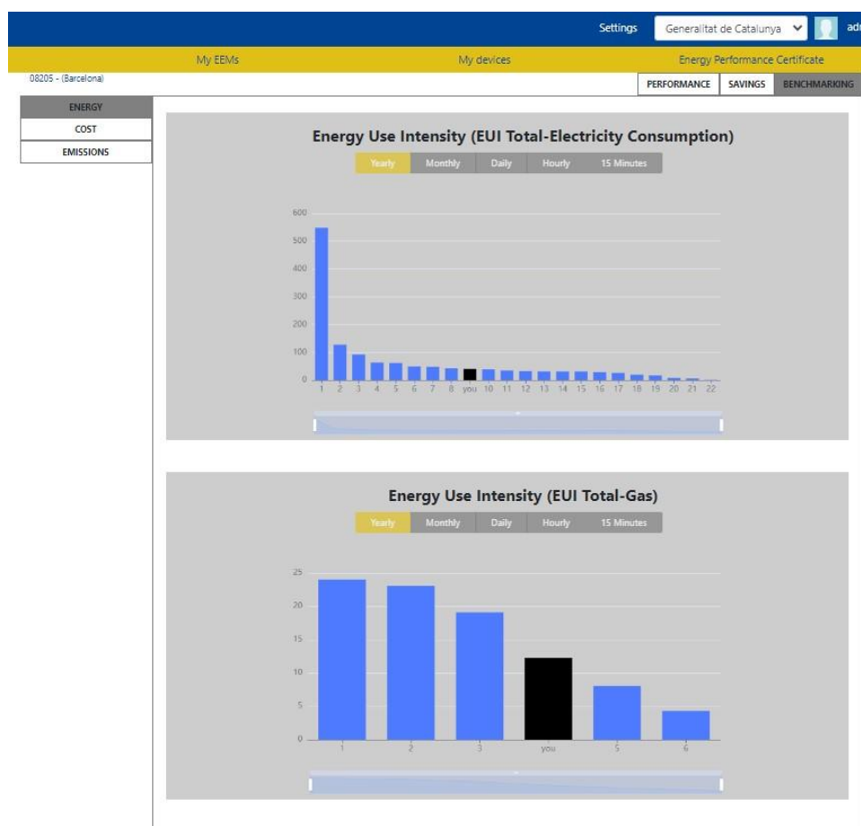
Figure 4. UC1 building benchmarking functionality for Electricity (top) and Gas consumption (bottom)
