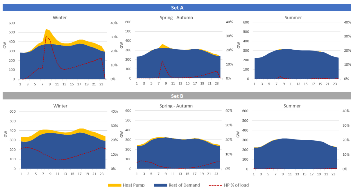
Figure 23. EU average seasonal hourly electricity demand profiles in Scenario 1 for Set A and B (hourly total and heat pump % share of total grid demand)
