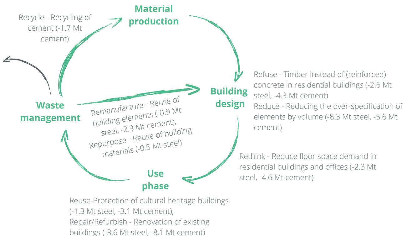
Figure 3: From a linear to a circular economy for buildings - Impact of individual actions on steel and cement [2] demand in EU buildings (Lotz et al. 2022b)
