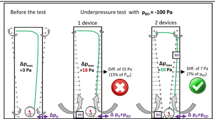
4.3 Two possibilities for **measuring the pressure deviation** [4]:
