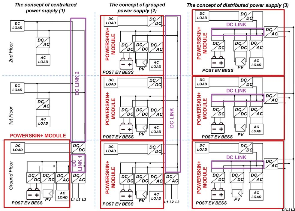
Fig. IV.5.2. Concepts for powering a non-residential building using POWERSKIN+ modules
