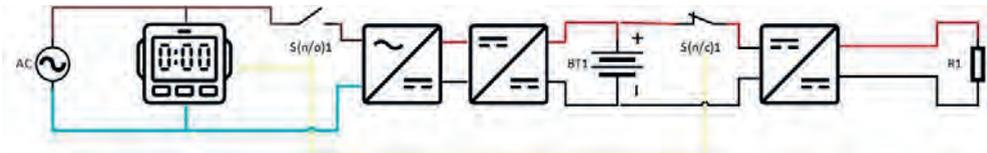
Fig. IV.5.6. Single line diagram of the battery energy storage microdemonstrator
