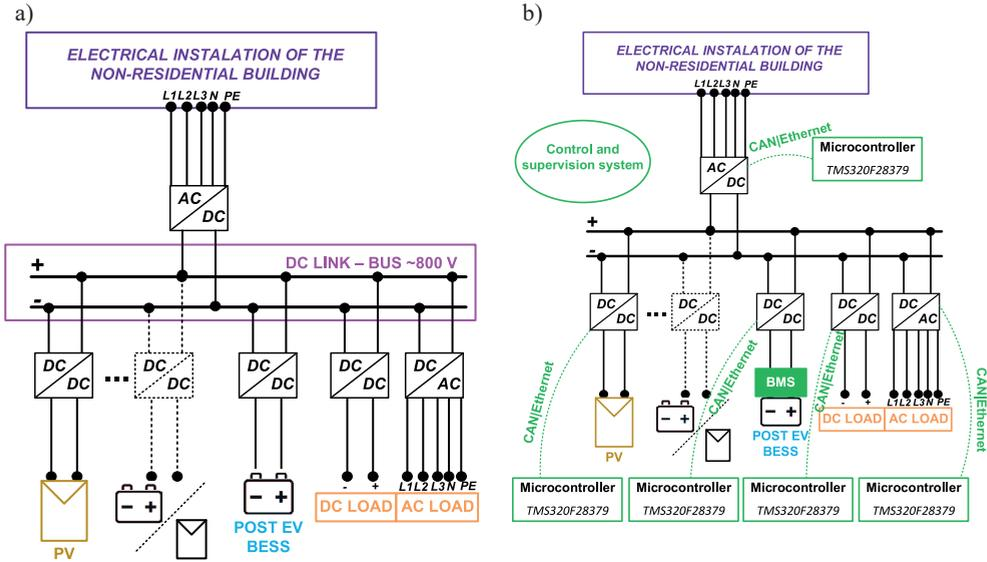
Fig. IV.5.3. Block diagram of the POWERSKIN+ module in the: a) electrical power part; b) communication part
