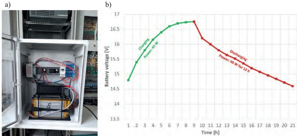
Fig. IV.5.7. Battery energy storage microdemonstrator for Politecnico di Torino: a) device; b)  $U(t)$  characteristics for charging and discharging processes
