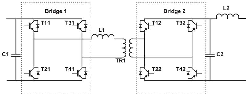
Figure IV.5.4. Topology of the dual active bridge (DAB) DC/DC converter – based on [16, 18]
