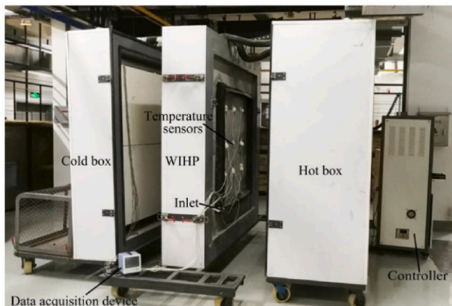
Fig. 10. Hot box apparatus used for the characterization of a Unidirectional Thermodiode with phase change. Source [95].
