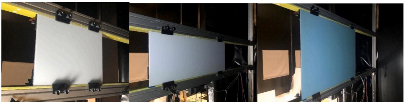
Fig. 9. The simulator set adjusted to host modules of different sizes and colours. From the left: six cells module, 12 cells module, 24 cells module.
