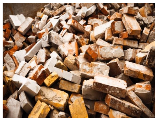
Figure 10 Preparing for re-use includes cleaning of bricks (Source: Danish Technological Institute)
