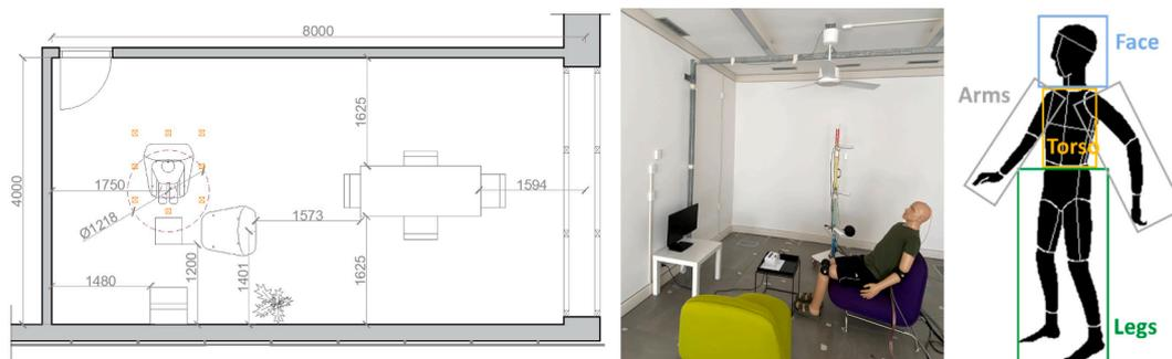
**Fig. 4.** Lab configuration for preliminary tests with thermal manikin.
