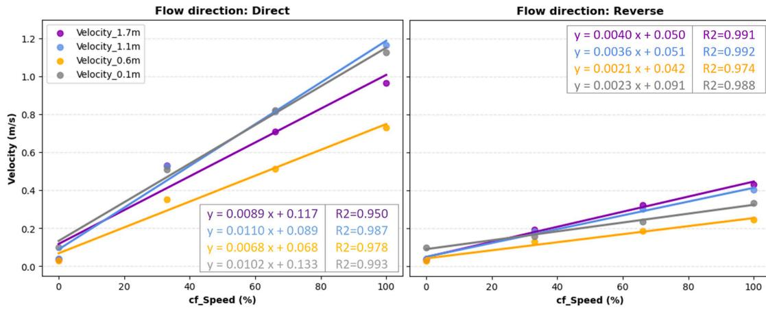
Fig. 5. The linear regression model of the average velocities at 4 height planes (1.7, 1.1, 0.6, and 0.1 m) for across fan speed (cf\_Speed: 0–100 %), where 100 % corresponds to 235 RPM in Direct mode and 195 RPM in Reverse mode, reflecting the actual operational characteristics of each flow direction.
