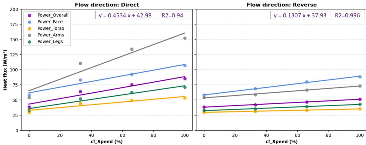
Fig. 6. The heat flux of the different parts of the thermal manikin for maintaining a constant skin temperature of 34 °C, for different fan speed (cf\_Speed) in both flow directions: Direct and Reverse. The linear regression model for the overall body is also reported.
