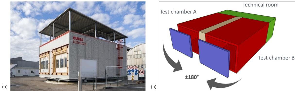
Fig. 2. Eurac Research's Facade system interaction lab (a) outdoor, (b) architecture (adapted from [33]).
