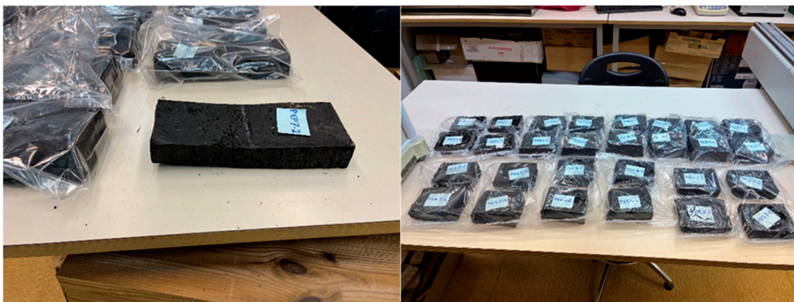
Figure 3. Test specimens for the measurements of flexural strength ( on the left ) and compressive strength ( on the right ).
